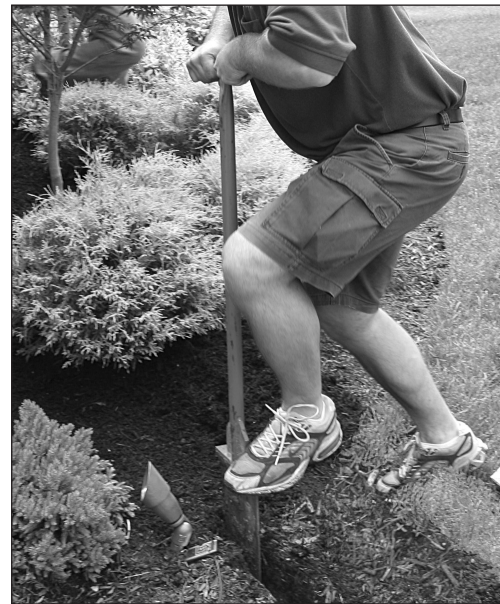
The CAST Trenching Tool (CWTT) cuts a narrow 8" deep trench ideal for laying wire.
