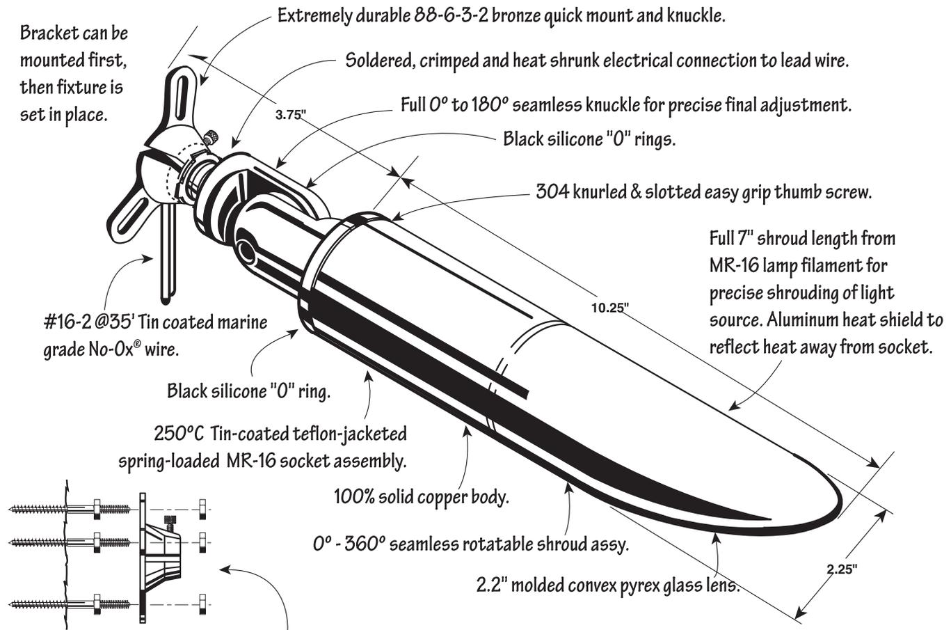
Mounting detail using CAST Tree Mount SS Hanger Bolts. (CTREEH1(24))
