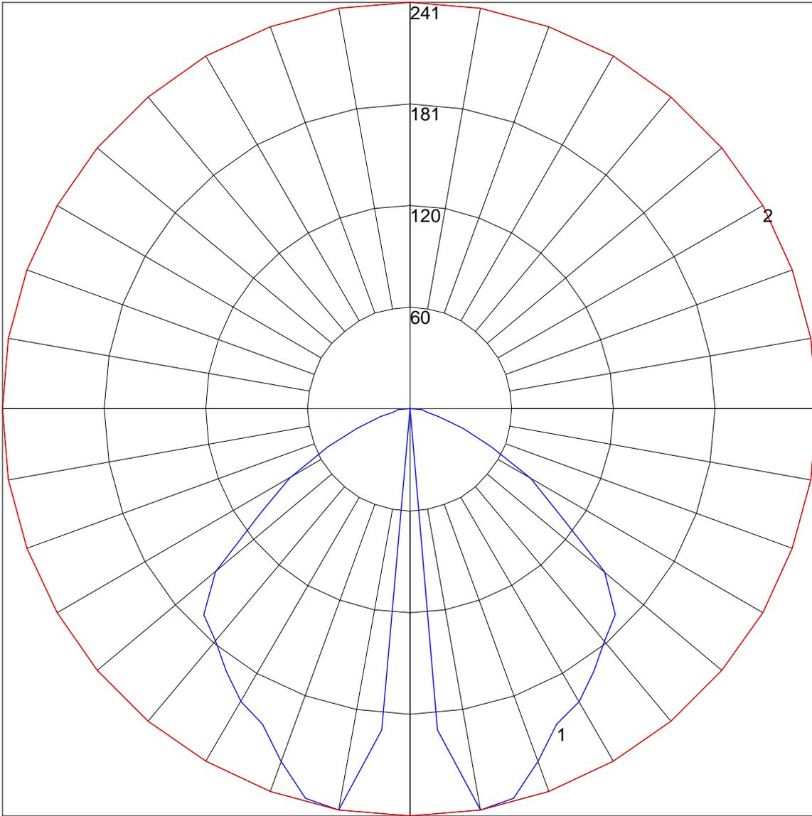
Maximum Candela = 240.85 Located At Horizontal Angle = 0, Vertical Angle = 10
