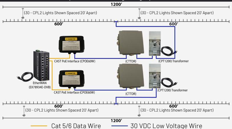
Using CAST Lighting PoE in concert with EtherWAN's 60W PoE Switch, you can now provide power from ONE switch. Power low voltage lights, cameras, access control, perimeter intrusion and tie into the network with one piece of equipment.
