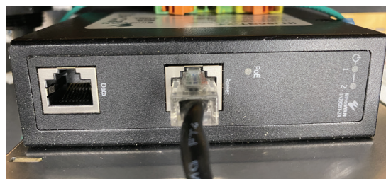
Typical router/injector switch, PoE++ by Etherwan
