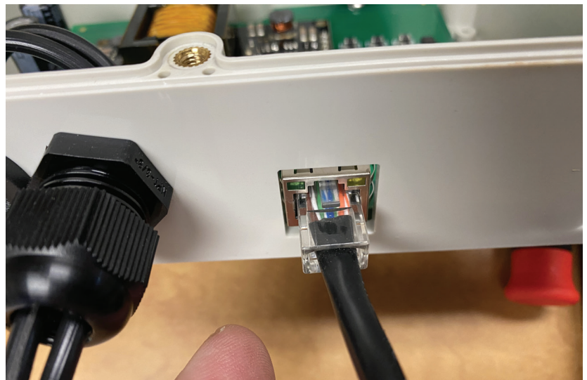
Attach Cat 5/6 cable from router switch/PoE++ to low voltage power supply model # CPOE60W
