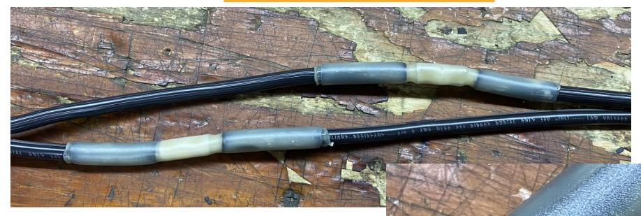
Heat Shrink when heated properly will release internal sealant which can be seen at the ends of the splice as shown.
