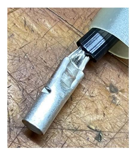
Use only a #8 AWG non insulated, Seamless, Tin Coated, Barrel, Butt Crimp, Splice Connection. LENGTH .832. I.D. of crimp cavity .181". OD of crimp .276"
