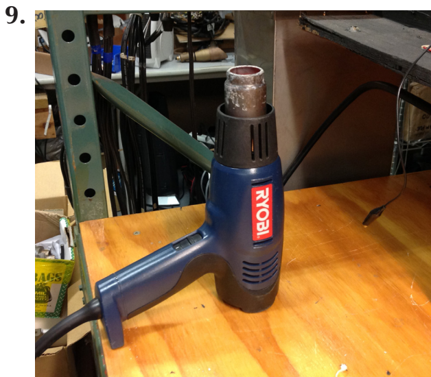
Typical Handheld Heat Gun. Warning: Never use an open torch to collapse heat shrink material as this will burn and crack heat shrink and cause corrosion and wire shorts.
